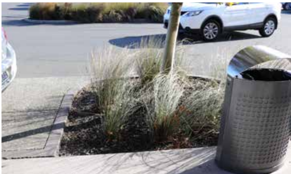
Use street furniture (e.g. a rubbish bin) to divert pedestrians around a tree pit. Location – Ansett Place Auckland
